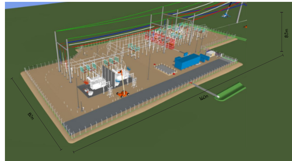
TYPICAL HIGH VOLTAGE SWITCHYARD (NOT TO SCALE)
