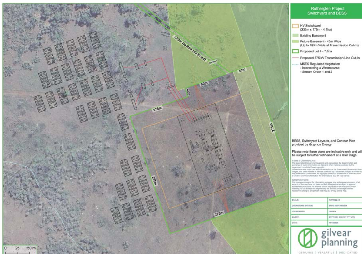
Figure 2: Rutherglen Project BESS and Switchyard Site Plan
