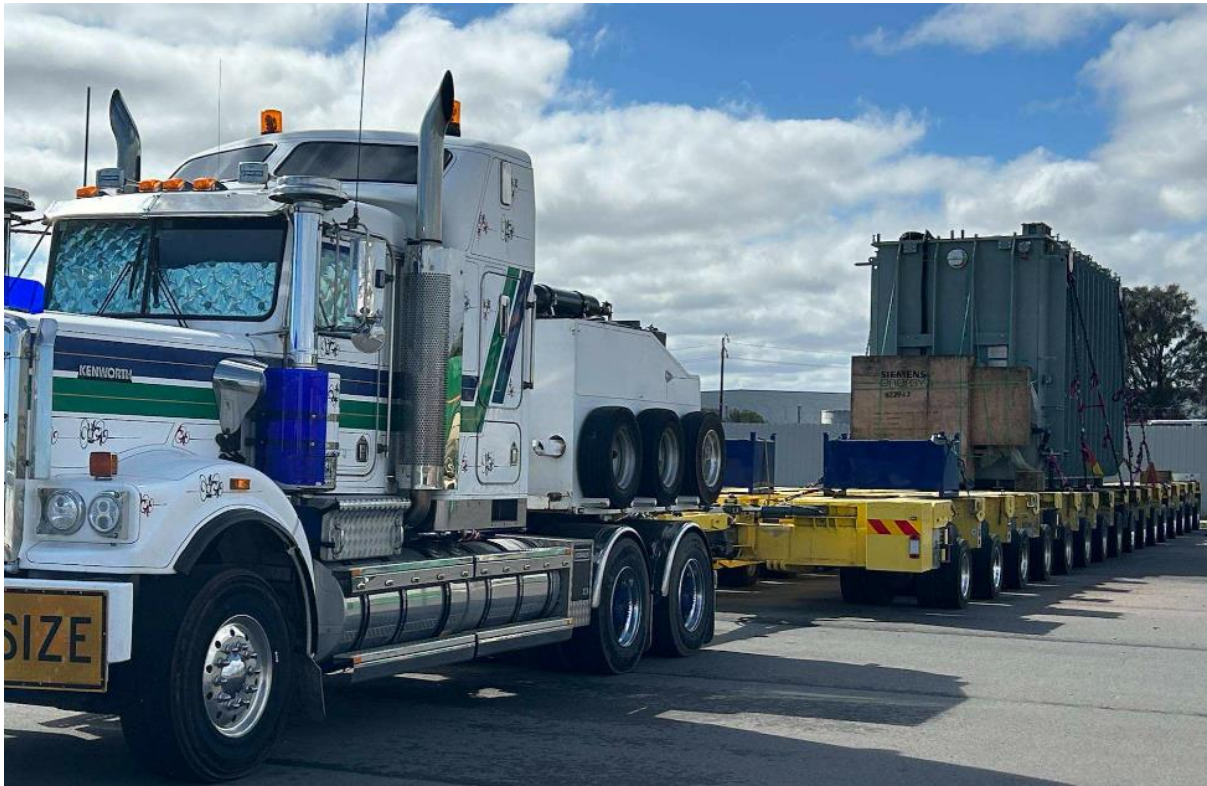
Photo showing the transformer loaded on the truck ready for delivery.
