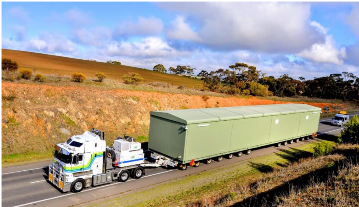
Example of a similar switch room delivery.
